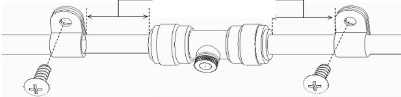
4. Secure the hose using the supplied Cable Clamps and screws.
